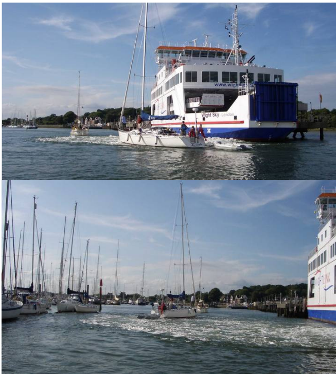
Figure 13: Effect of Thruster Slipstream on Passing Leisure Craft
