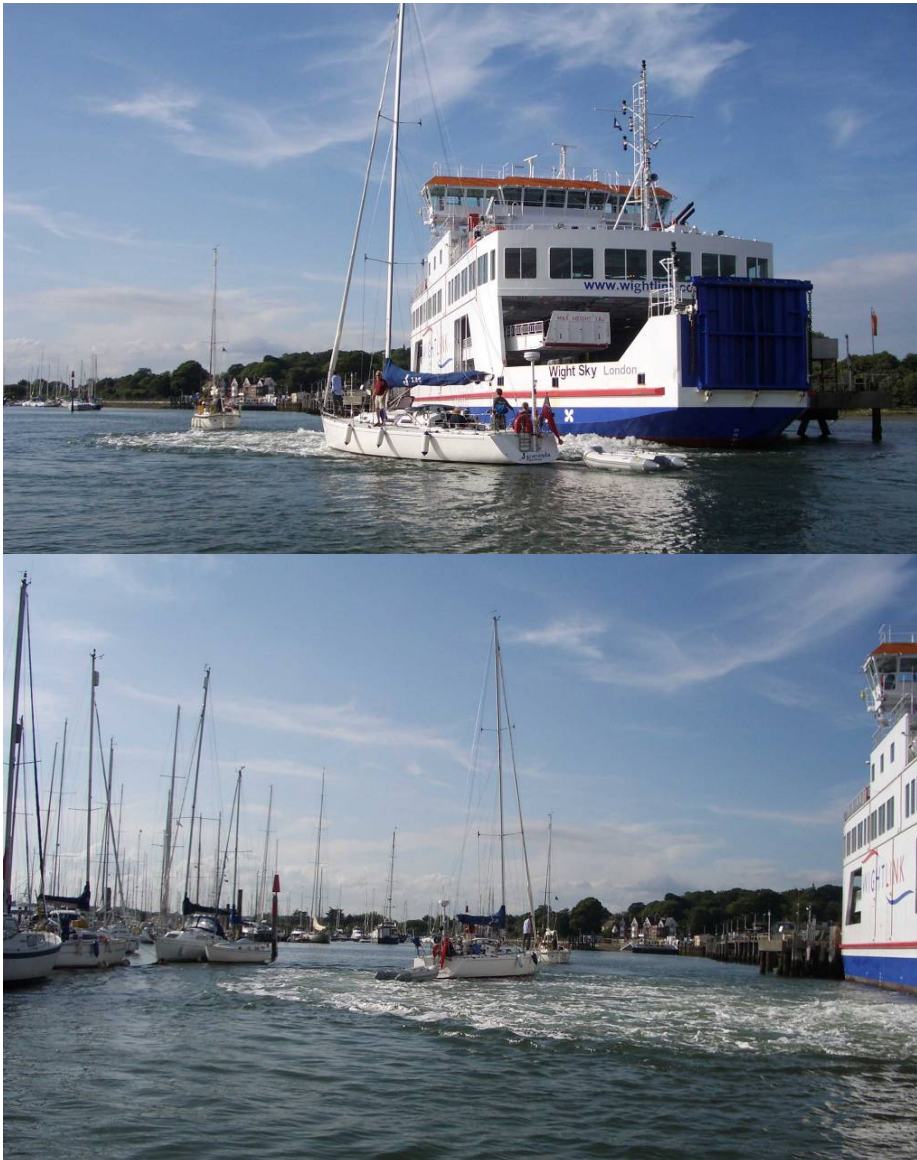
Figure 28: Effect of Aft Thruster Slipstream during Ferry Berthing.
